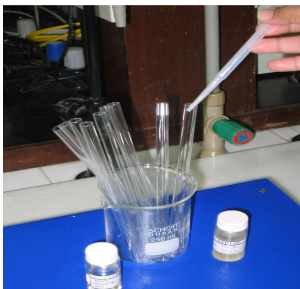
Figure 2: Samples prepared in the NMR tubes
