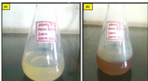
Figure 2: (A) 1mM AgNO 3 solution without plant extract and (B) 1mM AgNO 3 solution with Neem leaf extract after 2 hours
