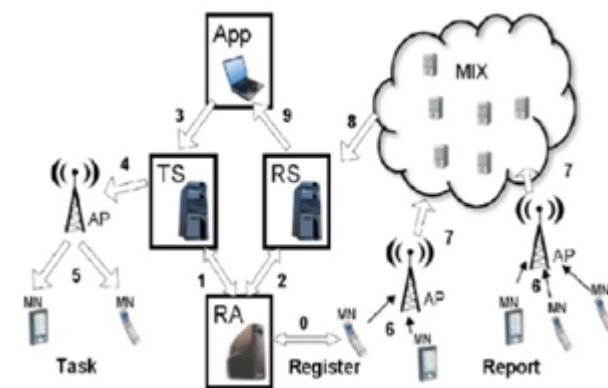
Figure 1: The AnonySense architecture and overview of the communications model.
