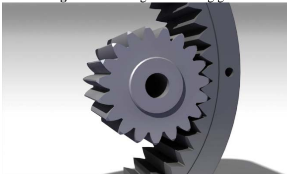
Figure 5: Close view Planet gear and Ring gear teeth meshing
