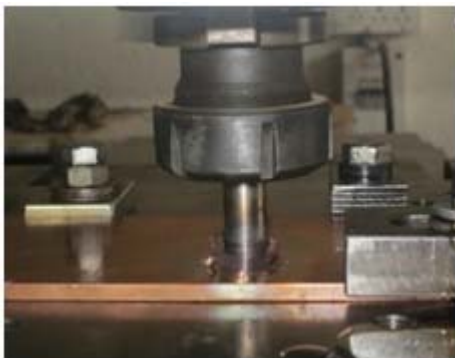
Figure 2: Friction Stir Surfacing on Copper
