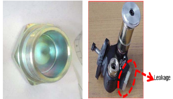
Figure 3: Base plug & Base plug leakage
