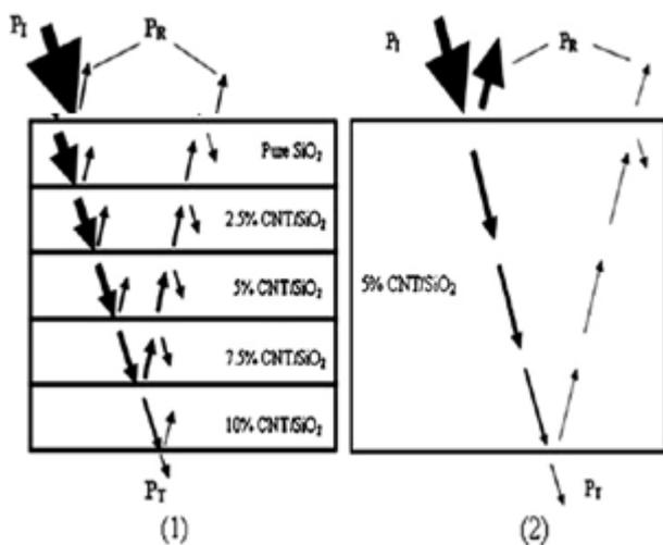
**Figure 9:** Schematic diagram of the incidence, reflecting and transmitting of the electromagnetic wave through the CNTs/SiO<sub>2</sub> composite materials: (1) multilayered sample (2) single layered sample [3]
