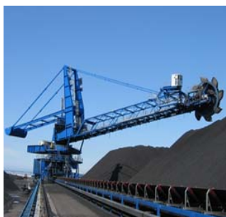
Figure 1: Stacker cum reclaimer in coal yard
