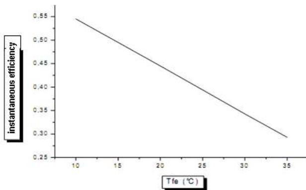
**Figure 9:** Variation of the instantaneous performance against the inlet temperature of the coolant
