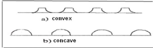
Figure 3: Geometric shapes of absorber plates
