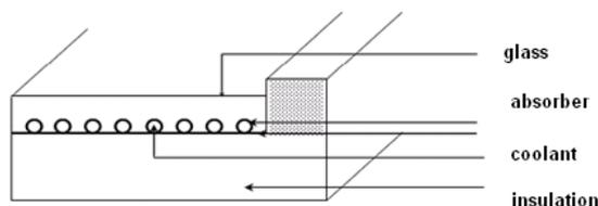
**Figure 1:** Components of a solar plane.
