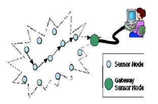
The WSN is built of "nodes" – from a few to several hundreds or even thousands, where each node is connected to one (or sometimes several) sensors. Each such sensor network node has typically several parts: a radio transceiver with an internal antenna or connection to an external antenna, a microcontroller, an electronic circuit for interfacing with the sensors and an energy source, usually a battery or an embedded form of energy harvesting.
